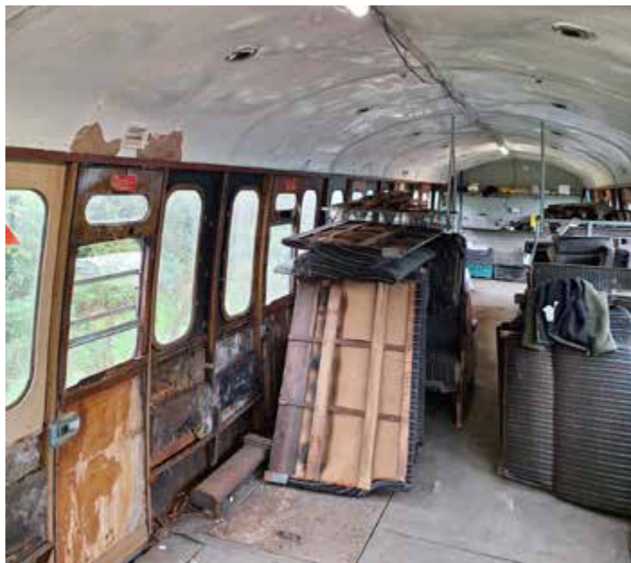
The interior of 14352 showing the lighting now in situ and the stripped out interior components sorted and stored. Photo Ashley Saunders
